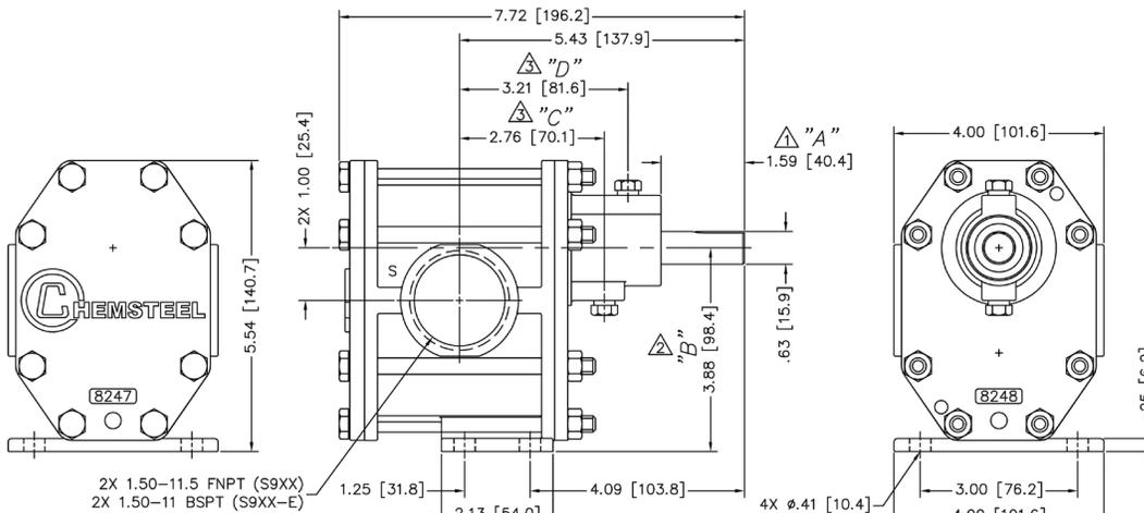
① DIMENSION "A" IS APPROXIMATELY 1.26 [32.0] FOR PACKING PUMPS WITH PACKING NUT INSTALLED. DIMENSION "A" IS 1.54 [39.1] FOR LIP SEAL PUMPS.
