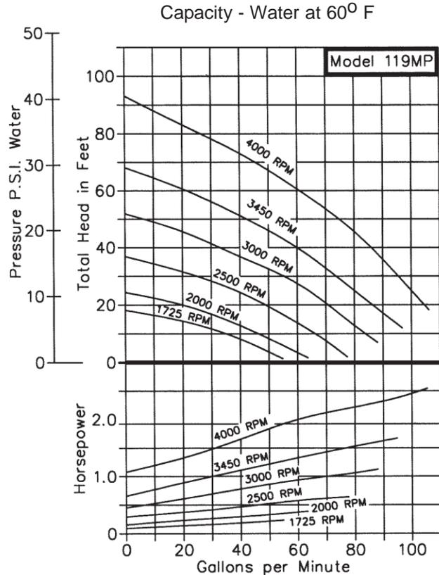
varies directly as flow and pressure. Maximum horsepower is required with a wide open discharge line. This is the point of maximum flow. With a throttled discharge, the flow decreased at a greater rate than the pressure increases thereby requiring less horsepower at the higher pressures. This is known as an "unloading" feature of the pump.
