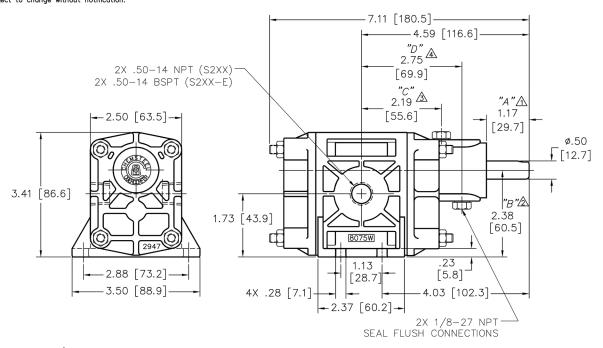
DIMENSION "A" IS APPROXIMATELY .84 [21.3] FOR PACKING PUMPS WITH PACKING NUT INSTALLED. DIMENSION "A" IS 2.25 [57.2] FOR LIP SEAL PUMPS.
