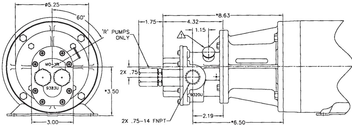
\*THESE DIMENSIONS ARE SPECIFIC TO A 56C OR 143TC/145TC FRAME MOTOR.
