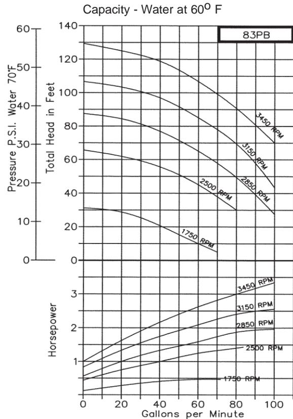
The height of the suction lift should be kept to an absolute minimum and the size of the suction pipe should be equal or larger than the pump inlet port. A foot valve with strainer is recommended at the beginning of the suction line. Self-priming centrifugals must be operated with the shaft in the horizontal position, regular centrifugals may be operated with the shaft horizontal or vertical.
