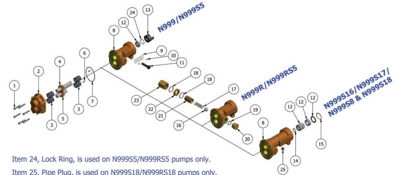
Item 24, Lock Ring, is used on N999S5/N999RS5 pumps only.
