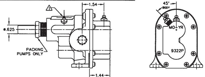
▲ GREASE FITTINGS (ITEM 17) INSTALLED INTO .125-27 NPT CONNECTIONS.
