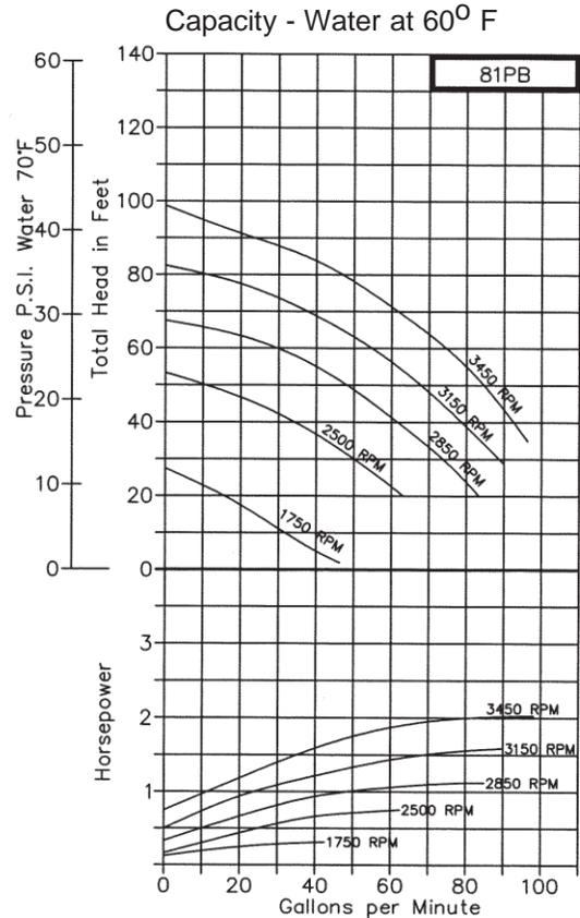
The height of the suction lift should be kept to an absolute minimum and the size of the suction pipe should be equal or larger than the pump inlet port. A foot valve with strainer is recommended at the beginning of the suction line. Self-priming centrifugals must be operated with the shaft in the horizontal position, regular centrifugals may be operated with the shaft horizontal or vertical.
